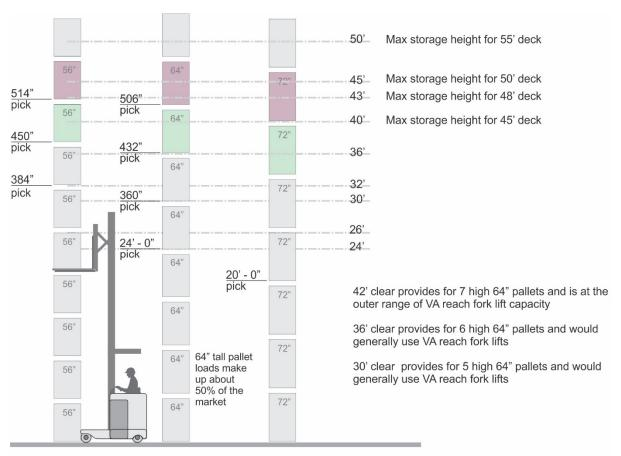
NA Reach trucks operate around 400" to 500" pick heights and use 108" to 120" aisles VNA Lift trucks operate in 400" and higher and use 60" to 72" aisles
